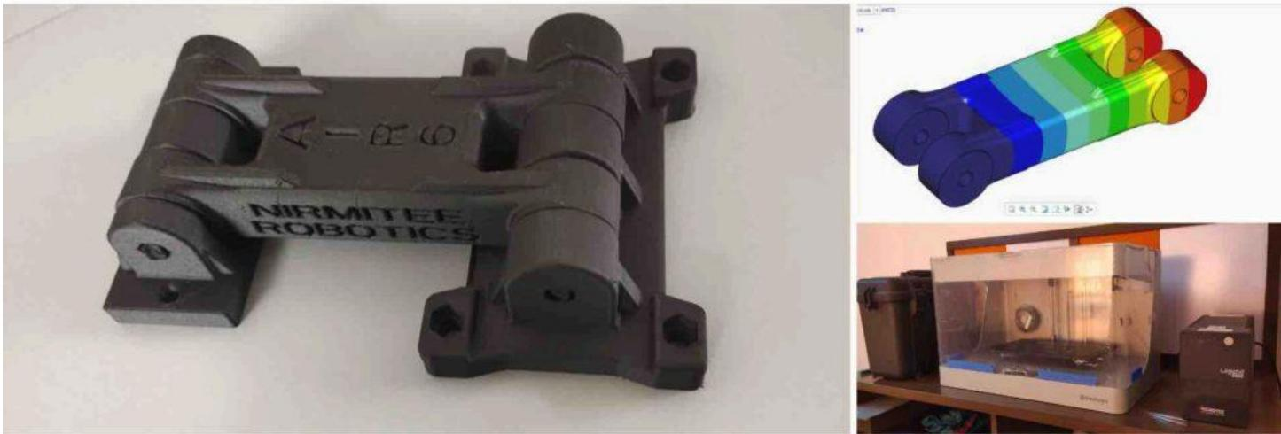
*Fork-end assembly used to lift robot arm designed and 3D printed by MRO Engineering using Markforged Mark Two Composite 3D printer/Source: MRO Engineering and Supplies*
