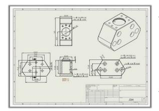
These drawings typically include detailed dimensions, tolerances, and other information necessary for the production process, such as material specifications and assembly instructions. They may also include information about surface finish, hardware, and other features
